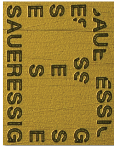
Fig 13 Amazingly, the repeat word 'SAUERESSIG' forming the letter 'B' is a mere 100µm in height, while the entire letter 'B' is just one millimetre tall. Image © Saueressig Ltd
