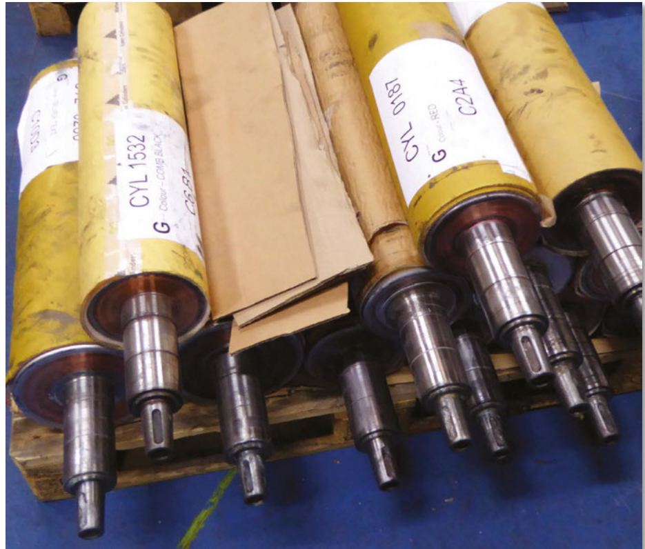
Fig 5 Cylinder deliveries back from the printers, covered with grease and ink and awaiting processing
