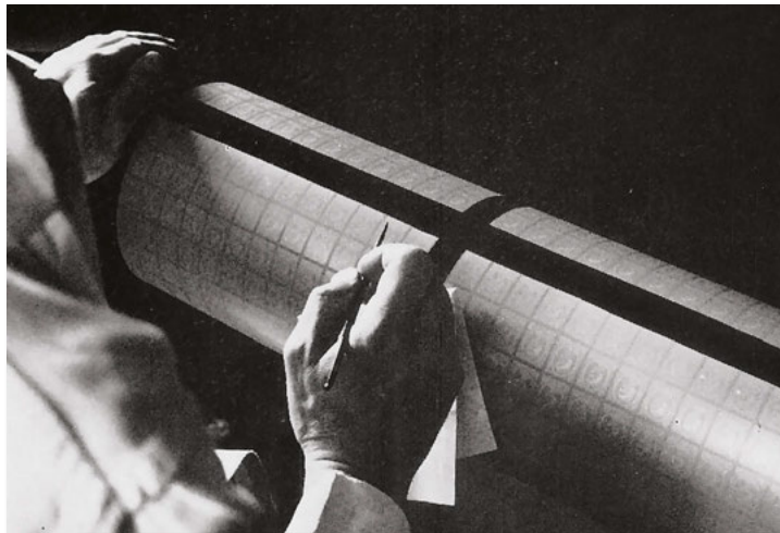
Fig 15 Painting over areas not to be etched at Harrison, early 1960s
