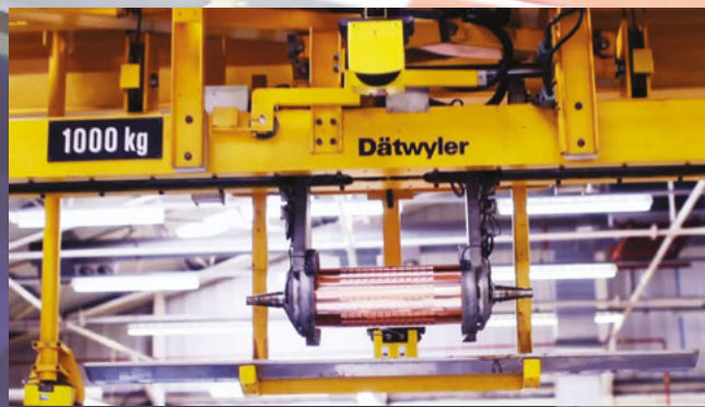
Fig 2 The first ever Daetwyler multi-tasking robotic crane system is in use to ensure maximum use of automation. Image © Saueressig Ltd
