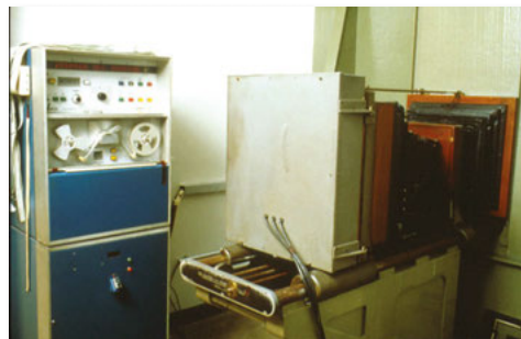
Fig 10 A 'step and repeat' camera showing a paper tape system for positioning each image correctly. Harrison, c1973
