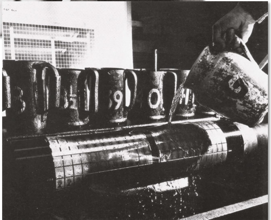
Fig 16 Preparing a gravure cylinder by hand-etching with varying strengths of acid
